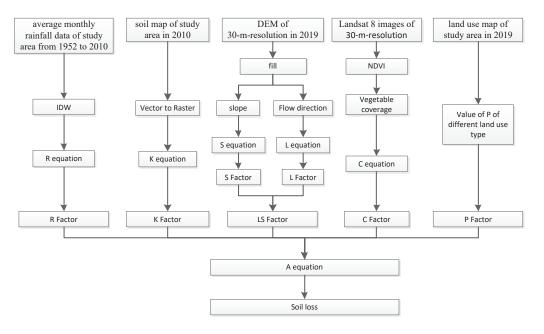
Fig. 2 The technical route of calculating soil erosion. Source: own elaboration
