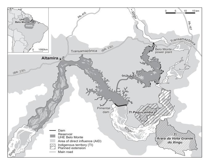
*Fig.* 1 The Belo Monte power plant complex. The river is dammed by the main dam (Pimental) and redirected via artificial channels to the Belo Monte power plant. Source: own elaboration based on ISA 2013: 46-47
