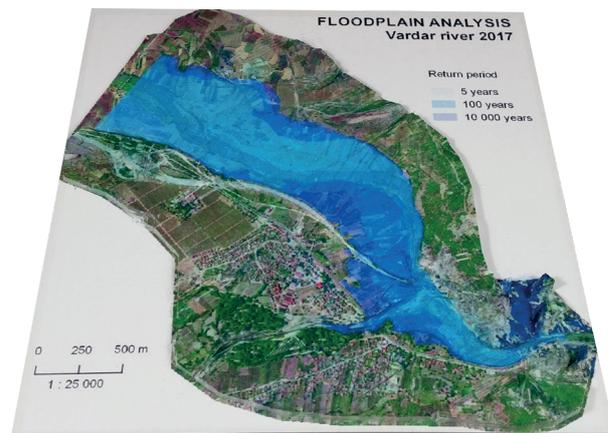
Fig. 5 True 3D printed model of the floodplain with transparent layers of return period isolines: a case study of the Vardar river. Source: own illustration
