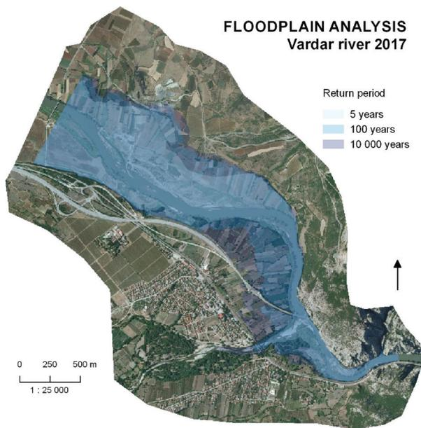
Fig. 4 Generalization of floodplain analysis with transparent layers and orthophoto of the Vardar river. Return water period of 5 years (1.319 km<sup>2</sup>), 100 years (1.756 km<sup>2</sup>) and 10,000 years (2.072 km<sup>2</sup>). Source: own illustration
