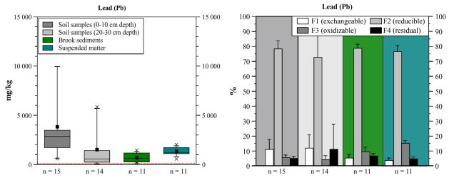
Fig. 5 The concentration of Pb in the soil (depth increments of 0-10 cm and 20-30 cm), sediment, and suspended matter samples: Boxplot diagrams (left side) represent the sum of all fractions (= total concentrations) (red line = precaution value for loam according to BBodSchV 1999: 1578). Bar charts (right side) represent the mean percentage proportions of the different fractions (F1 – F4) on the total concentrations (n = number of samples). Source: Own elaboration
