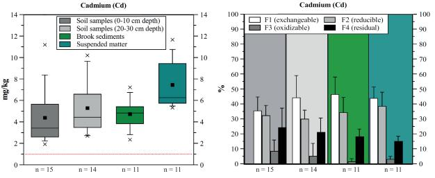
Fig. 3 The concentration of Cd in the soil (depth increments of 0-10 cm and 20-30 cm), sediment, and suspended matter samples: Boxplot diagrams (left side) represent the sum of all fractions (= total concentrations) (red line = precaution value for loam according to BBodSchV 1999: 1578). Bar charts (right side) represent the mean percentage proportions of the different fractions (F1 – F4) on the total concentrations (n = number of samples). Source: Own elaboration
