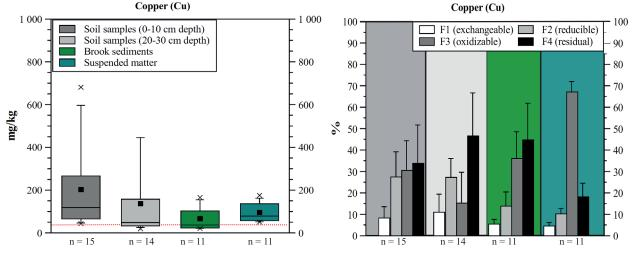
Fig. 4 The concentration of Cu in the soil (depth increments of 0-10 cm and 20-30 cm), sediment, and suspended matter samples: Boxplot diagrams (left side) represent the sum of all fractions (= total concentrations) (red line = precaution value for loam according to BBodSchV 1999: 1578). Bar charts (right side) represent the mean percentage proportions of the different fractions (F1 – F4) on the total concentrations (n = number of samples). Source: Own elaboration
