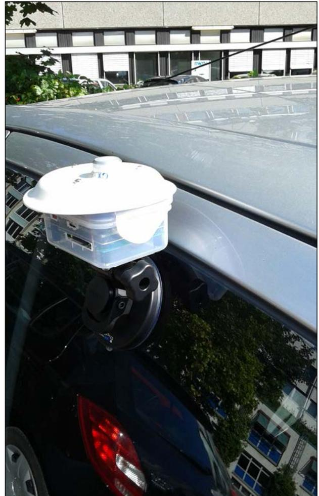
Fig. 5 Urbmobi 2.0 sensor installed on a car
